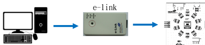
Figure 5.34 ESK-45F0062-S00 Programming Connection
