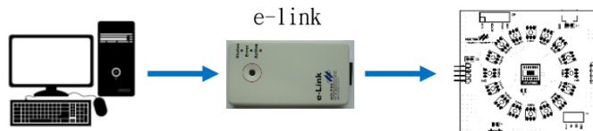
Figure 5.47 ESK-45F0063-S00 Programming Connection
