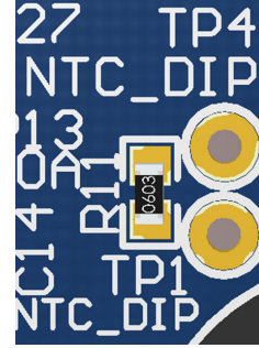
MOSFET Temperature Feedback Circuit Actual Component Layout and NTC_DIP Position
