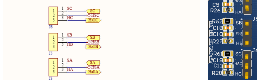
Sensorless and Hall Sensor Jumper Settings and Actual Component Layout
