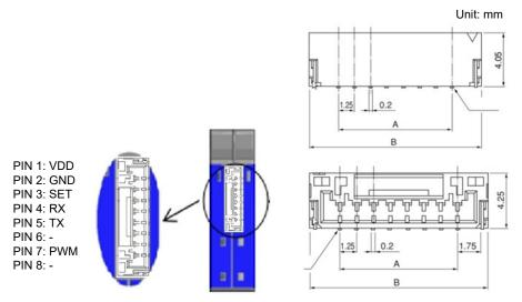
Terminal Description: JST-SM08B-GHS-TB-8P connector, pin spacing is 1.25mm, and pin number is 8.
