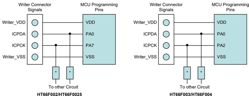
Note: \* may be resistor or capacitor. The resistance of \* must be greater than 1k or the capacitance of \* must be less than 1nF.
