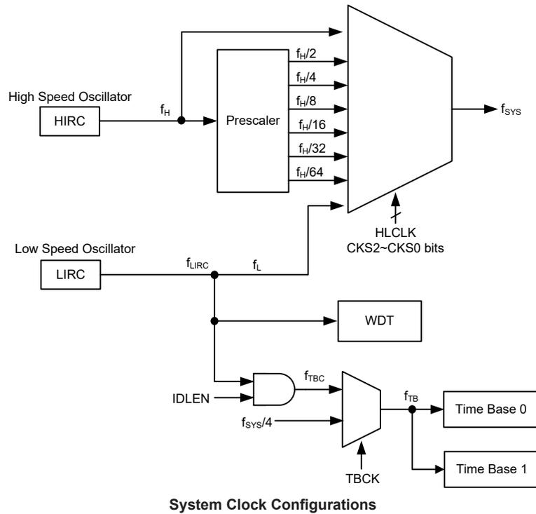
Note: When the system clock source  $f_{SYS}$  is switched to  $f_L$  from  $f_H$ , the high speed oscillation will stop to conserve the power. Thus there is no  $f_H \sim f_H/64$  for peripheral circuit to use.
