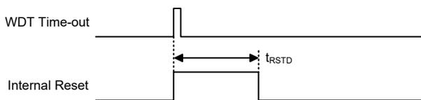
Note:  $t_{RSTD}$  is power-on delay, typical time=16.7ms
