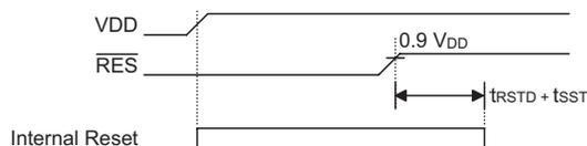
Note:  $t_{RSTD}$  is power-on delay, typical time=50ms
