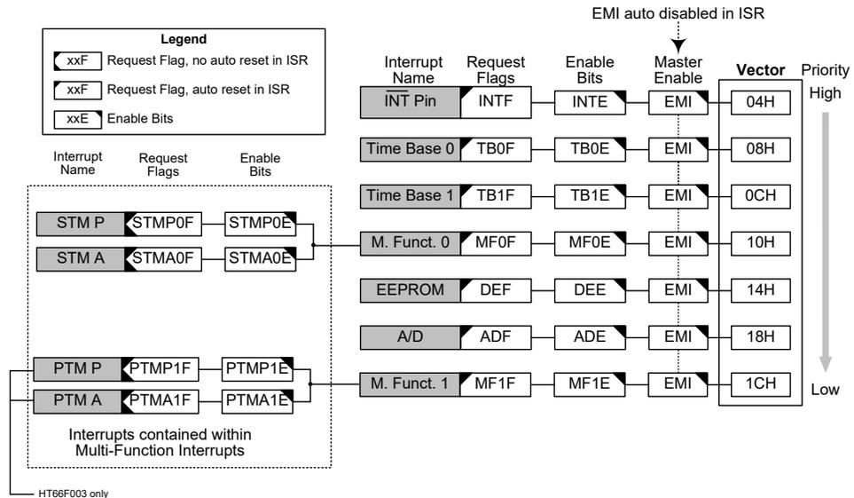
**Interrupt Structure – HT66F002/HT66F0025/HT66F003**
