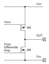
To keep power consumption to a minimum, the output short circuit current is limited to about -9mA for the source drive and 9.5mA for the sink drive. This is considered to be enough for most low power systems, however it is recommended only to used load resistors of >10k $\Omega$  for most applications. For heavy load driving applications, an external buffer stage using bipolar transistors is recommended.
