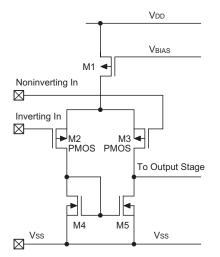
Since the input impedance of a PMOS transistor is inherently very high, they can be directly coupled to high impedance elements without loading effects. Examples could be coupling to ceramic transducers, integrating capacitors and resistor networks. It is this high input impedance characteristic that is its major advantage over its bipolar counterpart in certain application fields such as integrators where op-amp input currents can cause significant errors.
